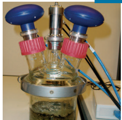
Verschiedene on-line-Sensoren zur optionalen Gasanalyse (CO 2 , CH 4 , ...) Optional gas analytic with different sensors (CO 2 , CH 4 , ...)
